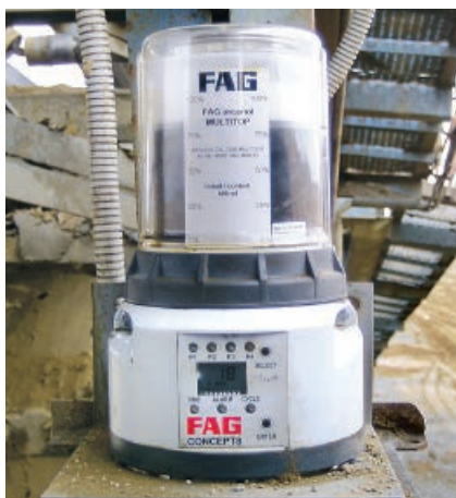
▲ FAG CONCEPT8 with Arcanol MULTITOP for belt tension pulley bearings
