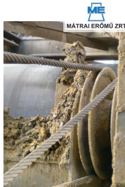
▲ Belt tension pulley for spoil conveyor belt
